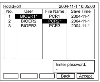
If the file has no password, press "Run" to enter file running interface or sample volume input interface. If the file has password, press "Run", a dialog box will be displayed for inputting the password. Press "Back" to go back the file list interface. Press "Accept" to confirm the password, and then the system will enter file running interface of sample volume input window.
