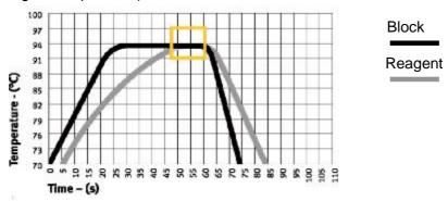
"Tube mode" has considered the phenomenon that the cooling & heating rate is a little slower than that of block. There is an overshoot after reaching the setting temperature, which can allow reagent to reach the setting temperature faster. During the same setting time as "Block", the actual time for reagent to keep the setting temperature is prolonged obviously. (Please refer to the following figure: relation between block temperature and reagent temperature)
